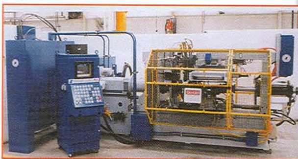
A 60 ton friction welder used to produce rear axle housings at 180 parts per hour with automated handling
